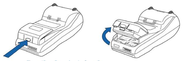
Figure 15 Removing the Smart Battery
